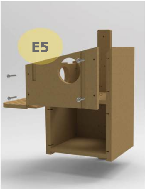
Screw Part E5 to Assemble Start with the back screws Line up the front screws to the slots before screwing
